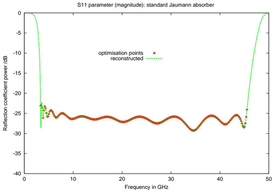
Figure 4: Predicted reflection coefficient of a multi-layer wideband circuit analogue FSS RAM.
