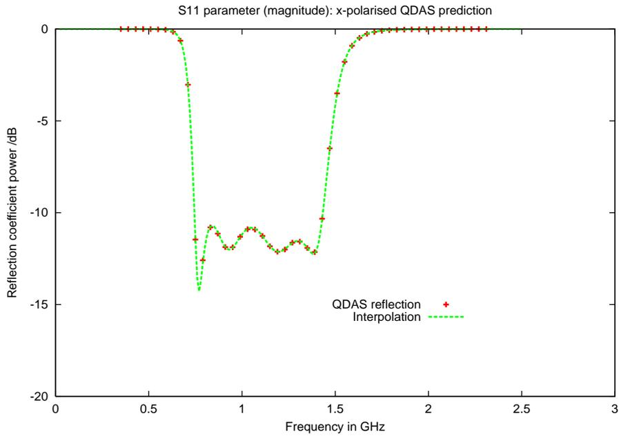
Figure 3: Predicted reflection coefficient of an electrically thin FSS RAM.
