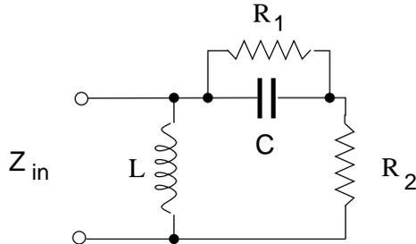
Figure 1: *Equivalent circuit for a thin capacitive FSS RAM.*
